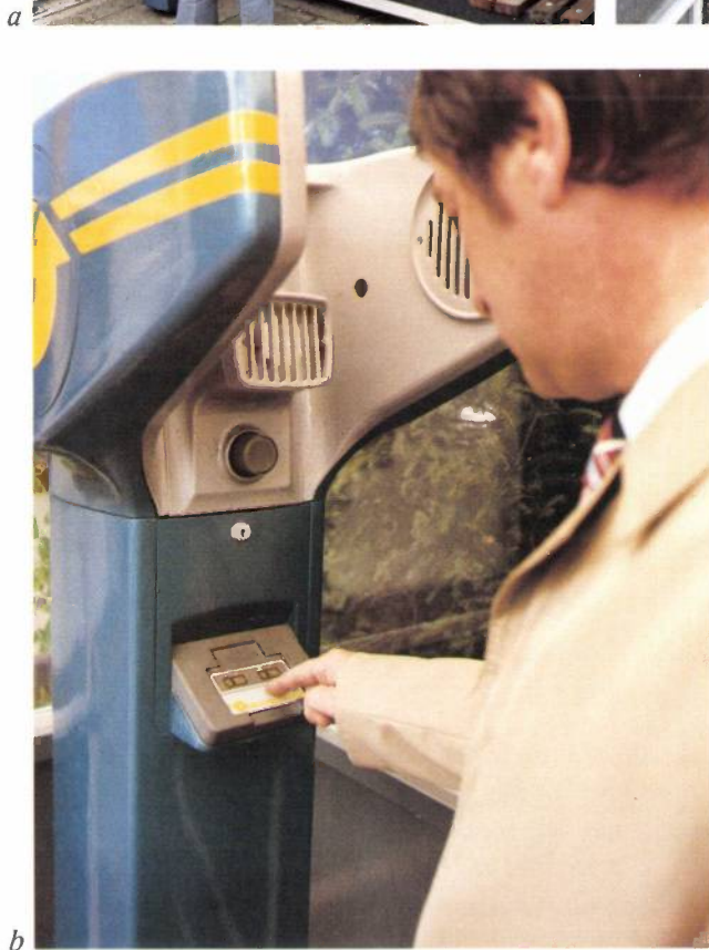
Fig. 2. a ) The passenger arrives at the O-BUS stop and selects the 'number' of his destination with the aid of the town map. b ) He puts his 'electronic card' on a small 'tray' and asks O-BUS control for transport. The reservation is made and the number of 'his' bus appears on the card. c ) An operator at control, who passes on passengers' requests to the computer system. d ) The bus arrives at the stop. Note that one bus may have several numbers which may change from stop to stop. e ) The driver's terminal in the bus. The driver receives route instructions from the control centre via the screen. f ) A display screen, based on liquid-crystal technology, for showing destinations inside the vehicle.
