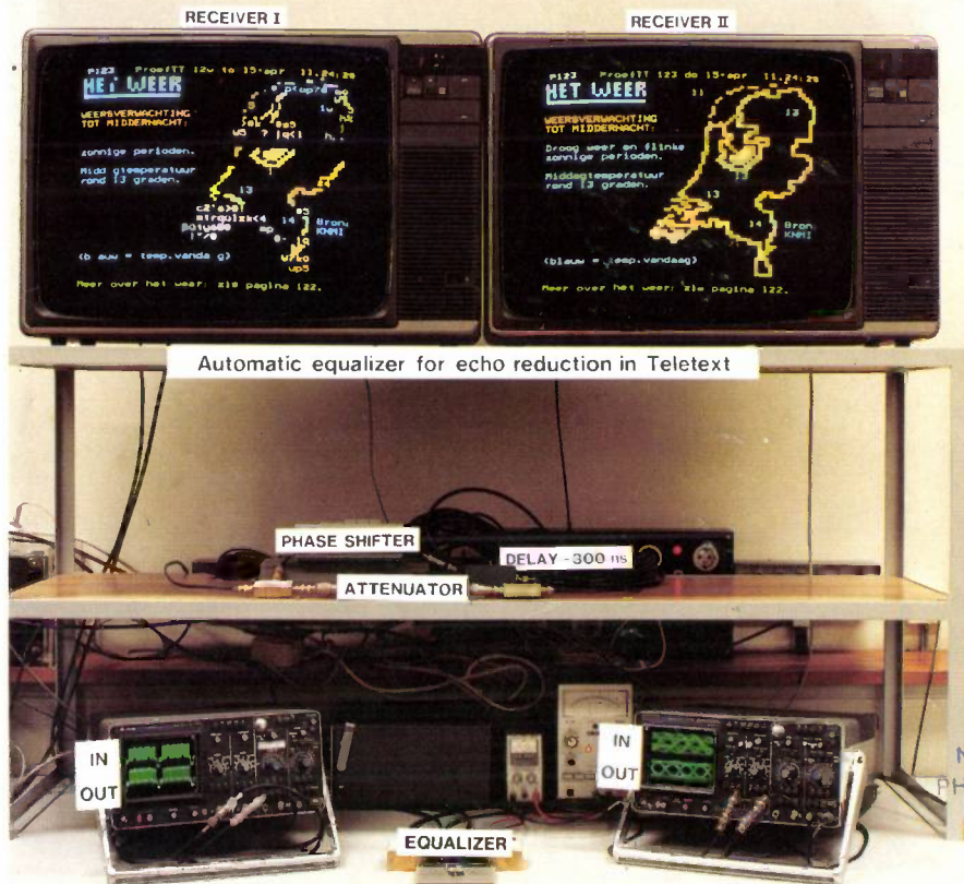
Fig. 4. Correction of the Teletext information by the equalizer. Receiver I : Teletext page degraded by the echo in fig. 3 . Many graphic elements of the test picture have been replaced by random alphanumeric characters. Receiver II : The Teletext page corrected by the equalizer. The oscillograms on the left show the time signals before and after the equalizer; those on the right show the eye patterns.
