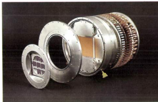
Fig. 4. The camera with top plate and window removed.
