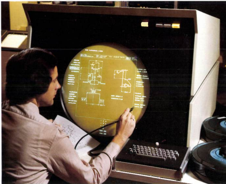
Fig. 1. Designing on an interactive display. The designer touches the light pen against a particular element on the display; this tells the computer that he is interested in that element. The element may be a piece of graphical information or an instruction; the result is either that data is retrieved from the data base, or that particular parts of the program are called. The designer can now take part in a dialogue with the computer.
