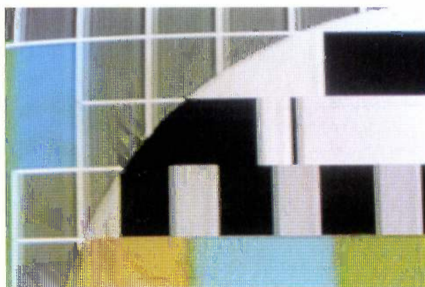
Fig. 3. Visibility in the test picture of an echo with a delay of 300 ns, an amplitude of 45% of the main signal and a phase angle of 0^\circ . Such echoes are not unusual and viewers do not find them particularly annoying.
