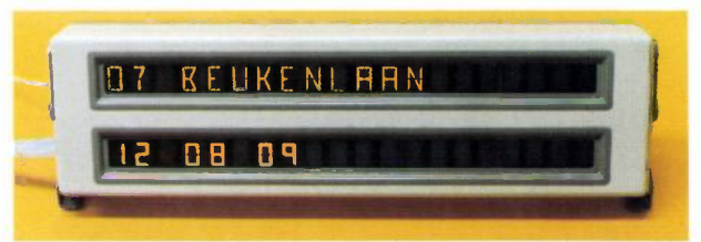
Fig. 2. a ) The passenger arrives at the O-BUS stop and selects the 'number' of his destination with the aid of the town map. b ) He puts his 'electronic card' on a small 'tray' and asks O-BUS control for transport. The reservation is made and the number of 'his' bus appears on the card. c ) An operator at control, who passes on passengers' requests to the computer system. d ) The bus arrives at the stop. Note that one bus may have several numbers which may change from stop to stop. e ) The driver's terminal in the bus. The driver receives route instructions from the control centre via the screen. f ) A display screen, based on liquid-crystal technology, for showing destinations inside the vehicle.
