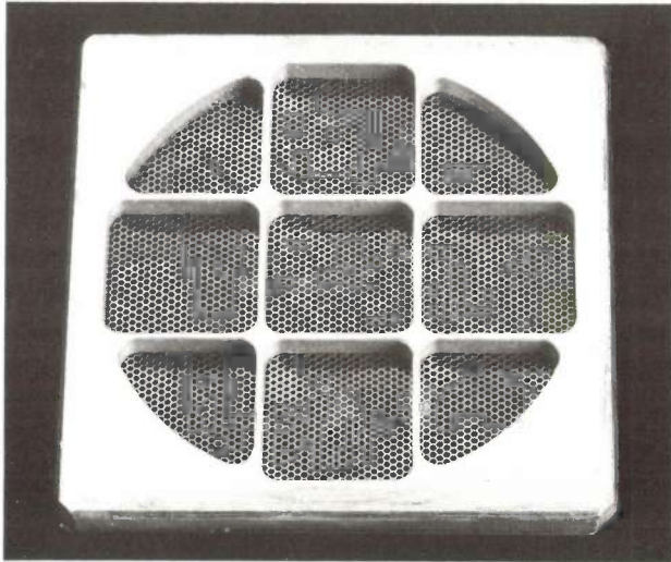
Fig. 6. The aluminium support grid with stainless steel meshes. The distance between the holes in the meshes is 1 mm. The meshes serve to support a nickel mesh (pitch 50 \mu\text{m} , thickness 5 \mu\text{m} ), which in turn supports the 'Lexan' film.
